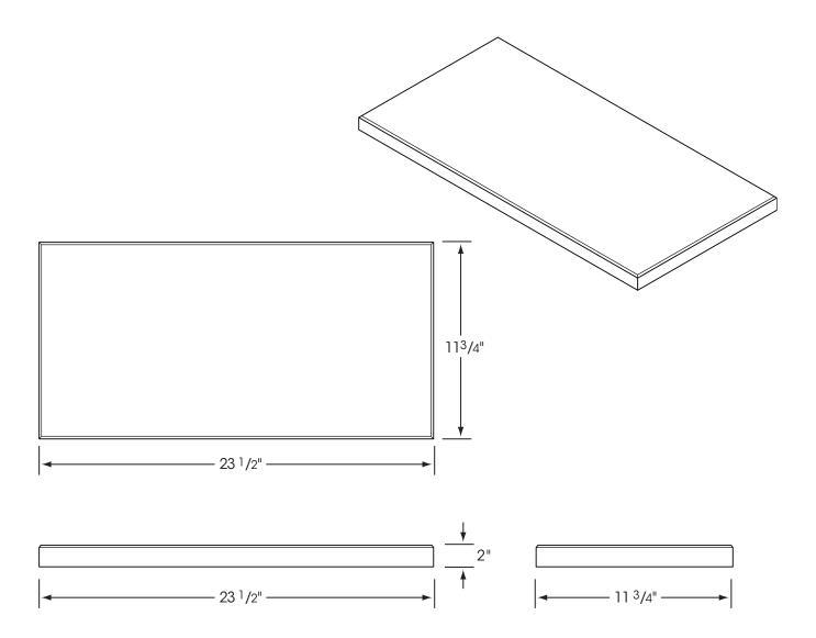
Thicknesses ranging from 1¼" - 3" are also available. A variety of dimensionally compatible sizes are available for installation with the 12" x 24" Paver. Contact Hanover® for a list of sizes.
