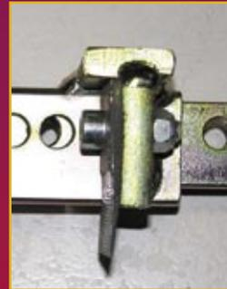
If the handles are set to close together, they will hit the stop-bar when squeezed. In this case full force can not be applied to the paver, pull out the **QUICKPIN** and reset the handles.
