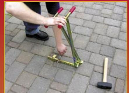
3. Next, insert the **QUICKPIN**. The holes on the slide and bar are offset for precise handle width. Select a width that allows both handles to be squeezed with one hand, but not too close. If too close, the handles will touch when force is applied and the operator will not get enough grip on the paver to remove it.
