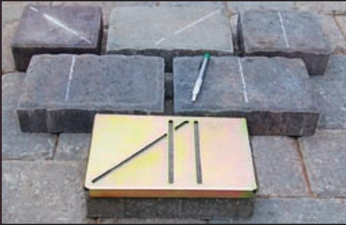
The 6 x 9 x 45° Marker is the newest addition to the template marking tools. It allows for quick and accurate marking of both 6" x 9" and 6" x 6" pavers. The 6 x 9 x 45° Marker allows following cuts:
