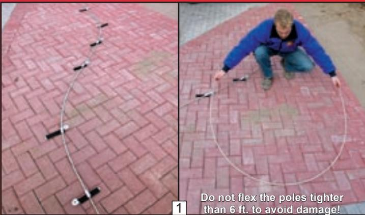
1 Do not flex the poles tighter than 6 ft. to avoid damage!
