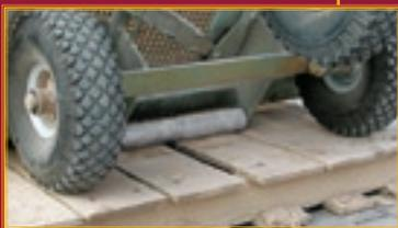
Sometimes less boards are used on the pallet tops (unlike this one), and one or both tires line up with the openings. The roller on the bottom allows the **PAVERCART** to still
