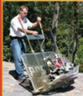
The optional **CARTTRAY** gives the **PAVERCART** more versatility. Easy to mount and dismount with one hand and no tools. Use to transport retaining wall blocks or plate tampers without wheel kits around the jobsite.
