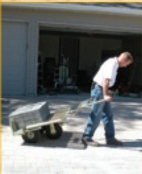
An optional Third Wheel kit is available for the **PAVERCART**. It bolts on directly below with operating lever. The Third Wheel eliminates the need for the operator to balance the cart. Some operators prefer to pull the **PAVERCART**, especially on rough terrain or going up steep grades.
