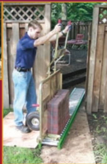
When gates are too small to fit the **PAVERCART** through, use a 10' roller conveyor with 10" wide rollers. Place the roller conveyor in the gate entrance and put a piece of plywood on the grass to reduce damage and prevent rutting.
