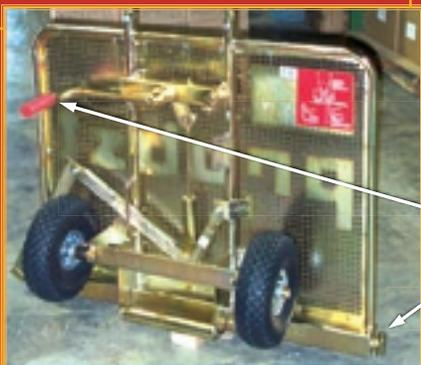
The operating handle has a simple but secure over-center cam action.
